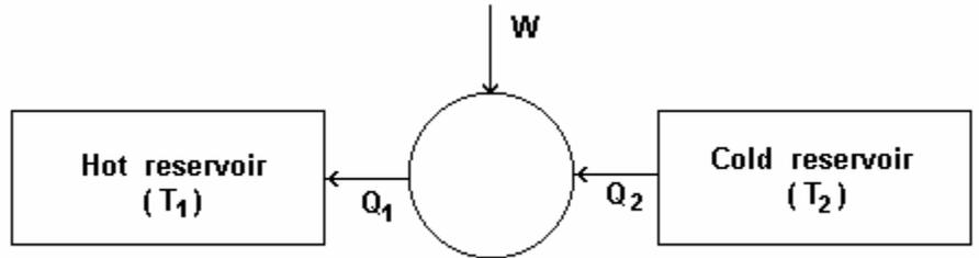
Schematic representation of a heat pump / refrigerator
