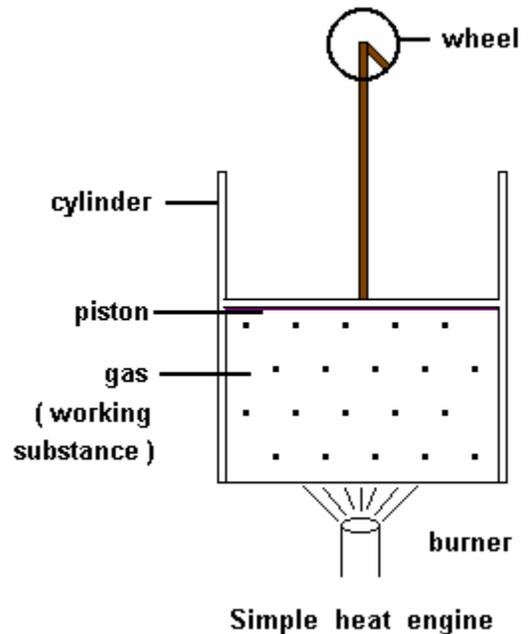
Here, gas is the working substance, burner is the heat source and the arrangement to release the gas and heat after expansion is the heat sink. The working of the engine is explained in the following schematic diagram.
